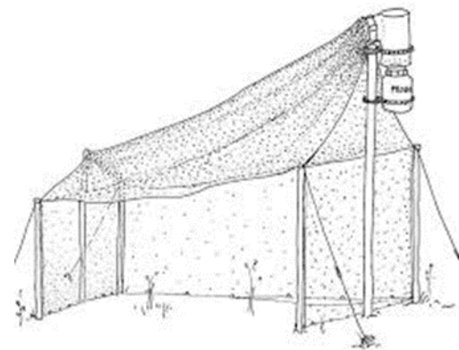
Figure 19: The Malaise trap is a large tent-like structure used to capture, kill and preserve flying insects, particularly Hymenoptera and Diptera. The trap is made of a material like PET mesh and can be in different colors.
